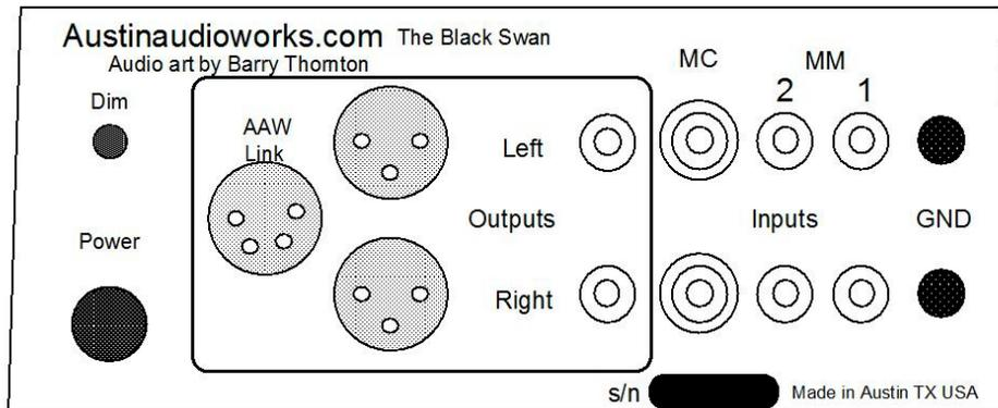
The Moving Magnet Cartridge (MM) feeds are via standard RCA type connectors. Two (MM) Cartridges can be accommodated and plugged into either Input 1 or 2. These are traditional SE (Single Ended) inputs. Loading is adjusted from the front panel.
