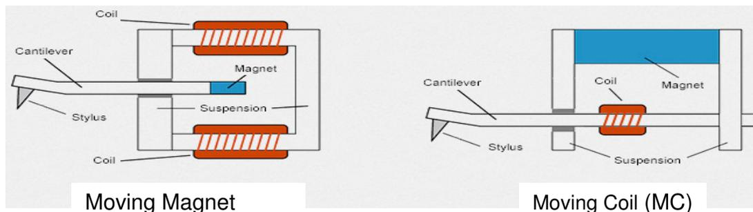
Because cartridge makers don't build preamps and vice-versa, some convention was needed for interfacing compatibly between the two, which became a standard loading guideline. For Moving Magnet (MM) it is 47 kohms with about 200-300 pf in parallel, for Moving Coil (MC) it is 100 ohms.
